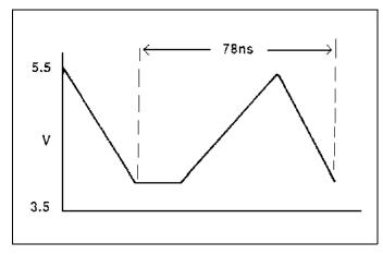
Figure 3 - Reference Oscillator (Input To U206, Pin 2)
