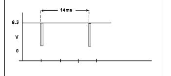
Figure 8 - S Data (Input To U206, Pin 12). (Radio In Scan On A Single Channel)
