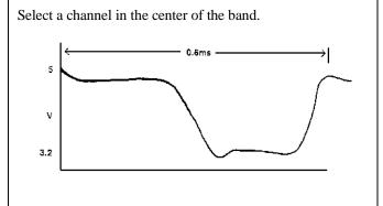
Figure 4 - FIN (Input To U206, Pin 10)
