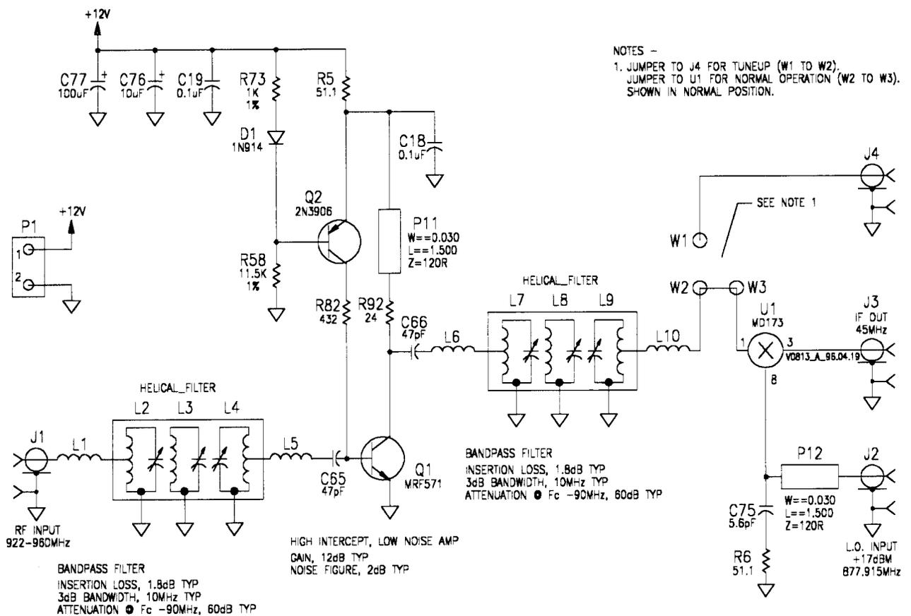
Figure 10-3 Front End Schematic
