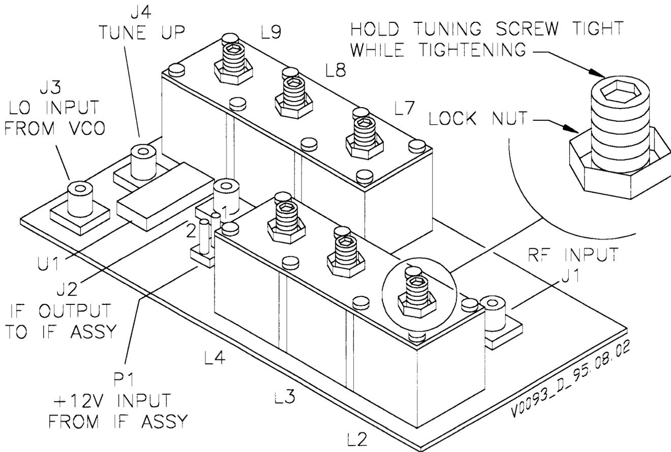
Figure 7-4 RF Assembly - Adjustments
