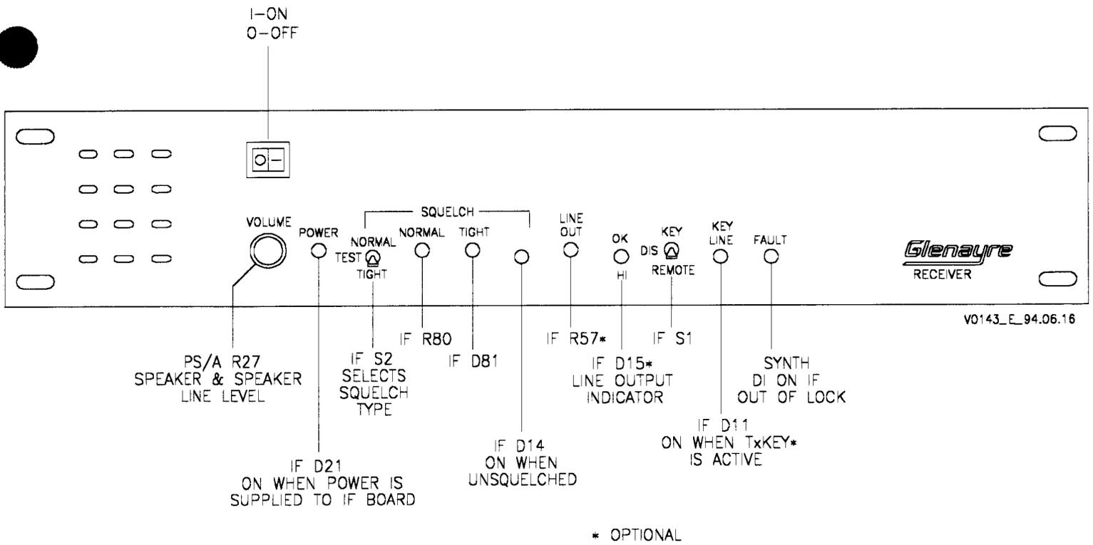
Figure 5-1 Front-Panel Controls and Indicators
