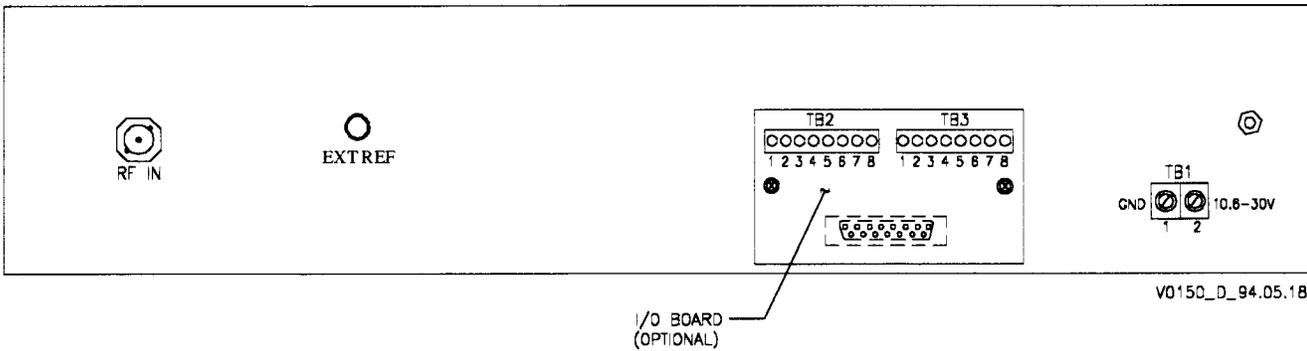
Figure 3-2 Receiver Rear View
