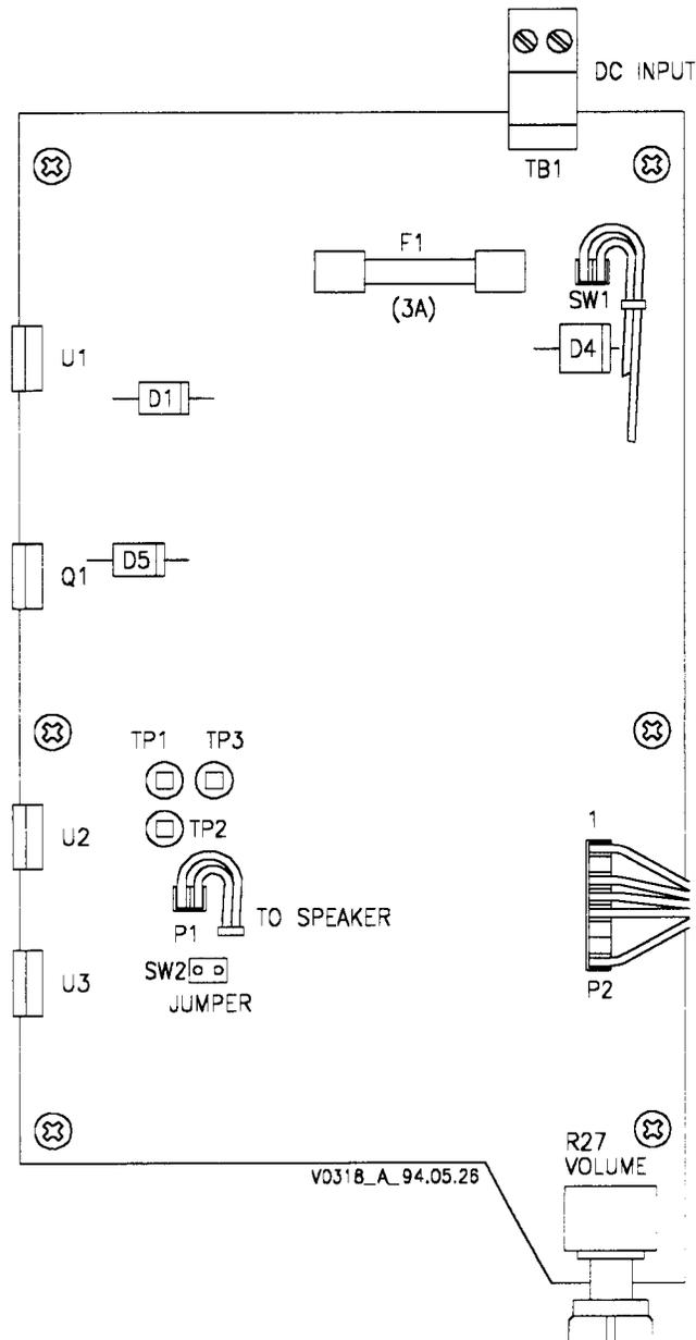
Figure 7-6 PS/A Board Controls and Indicators
