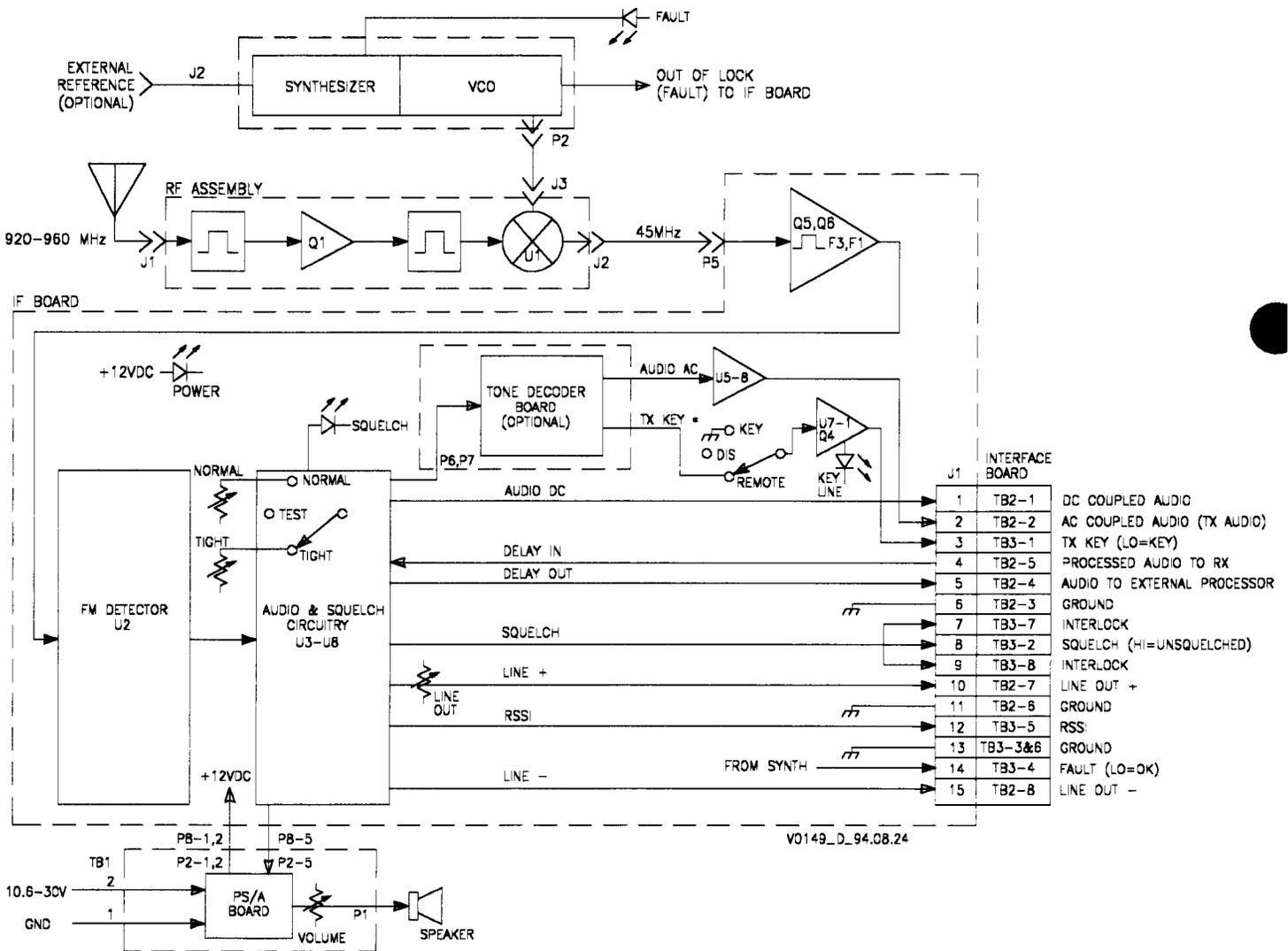
Figure 3-4 Receiver Functional Diagram
