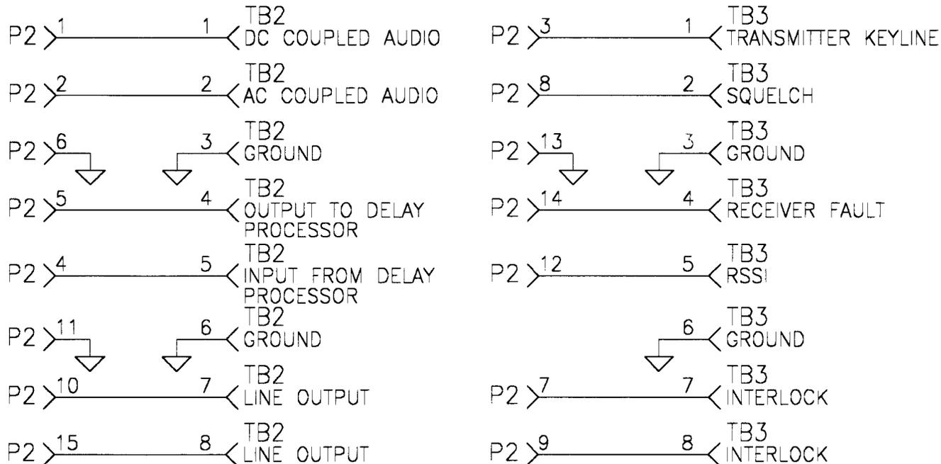
Figure 10-1 Interface Board 265-0305-002 Assembly and Schematic
