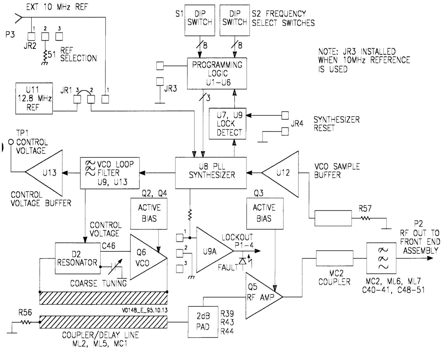
Figure 6-1 Synthesizer Functional Diagram
