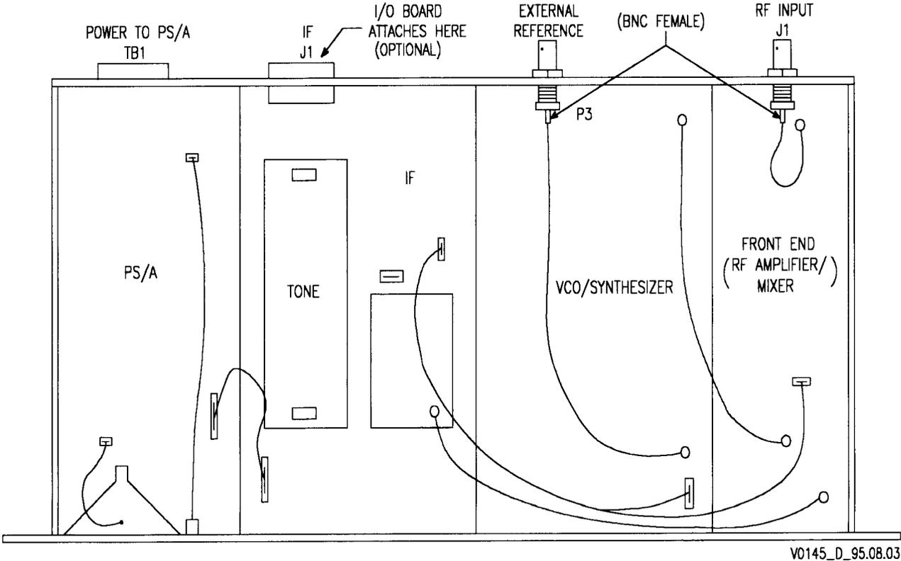
Figure 3-3 Top View of Internal Assemblies
