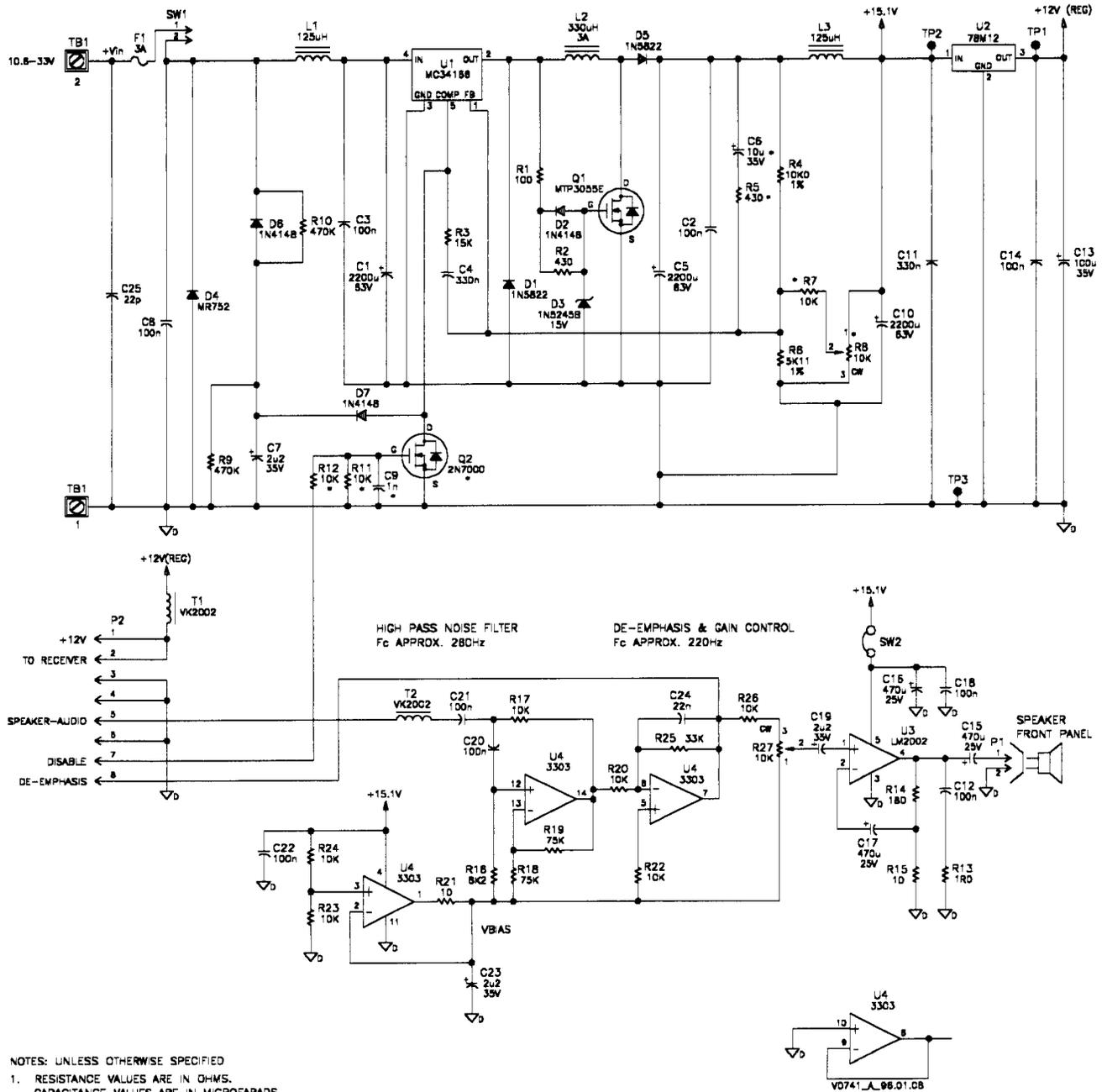
Figure 10-5 PS/A Board Schematic
