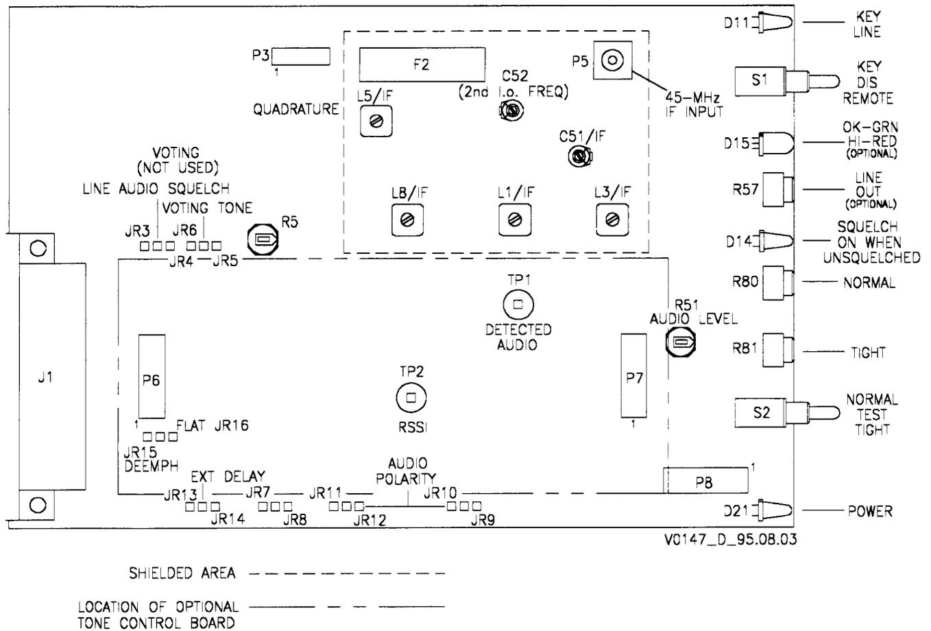
Figure 7-5 IF Board Controls and Indicators
