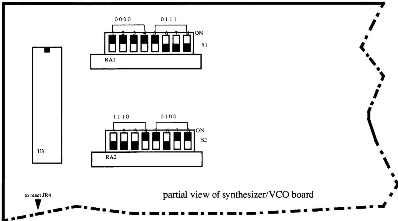
Figure 7-3 Programming Synthesizer Frequency
